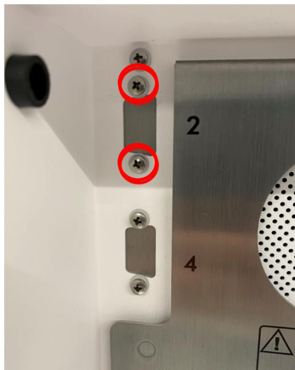
Figure 18. Left: opening the electronics compartment from the front side Right: Removing the plastic connector cover strip.
