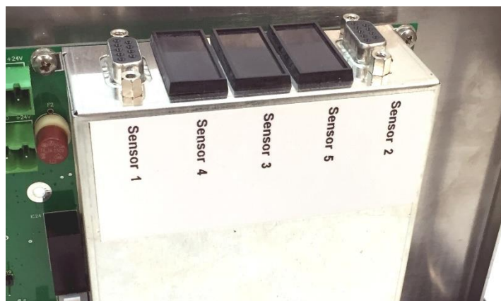
Figure 14. Control board with 2 sensor boards under the EMC enclosure.
