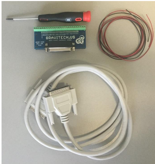
Figure 4. I/O connection set supplied with the DECADE Elite.
