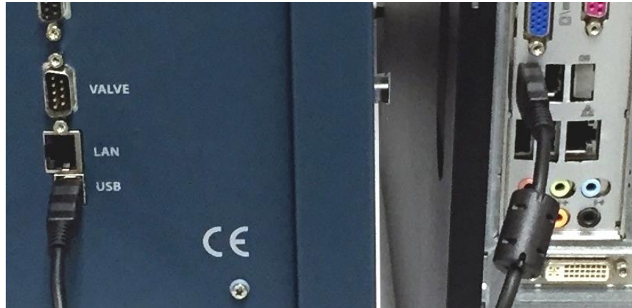
Figure 3. Left: rear panel DECADE Elite with USB cable connected (B type connector). Right: rear panel of the PC with USB cable connected (A type connector).
