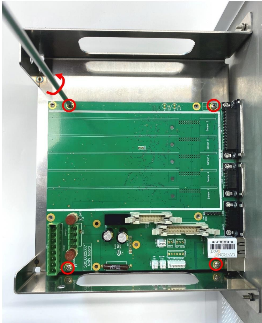
Figure 28. Remove M3 screws fixing the PCB on the PCB frame.
