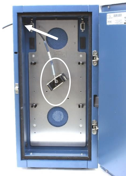
Figure 6. Take out flow cell and place temperature sensor within white circle and close the door. Insert the temperature probe via the tubing hole (arrow) and close the door.
