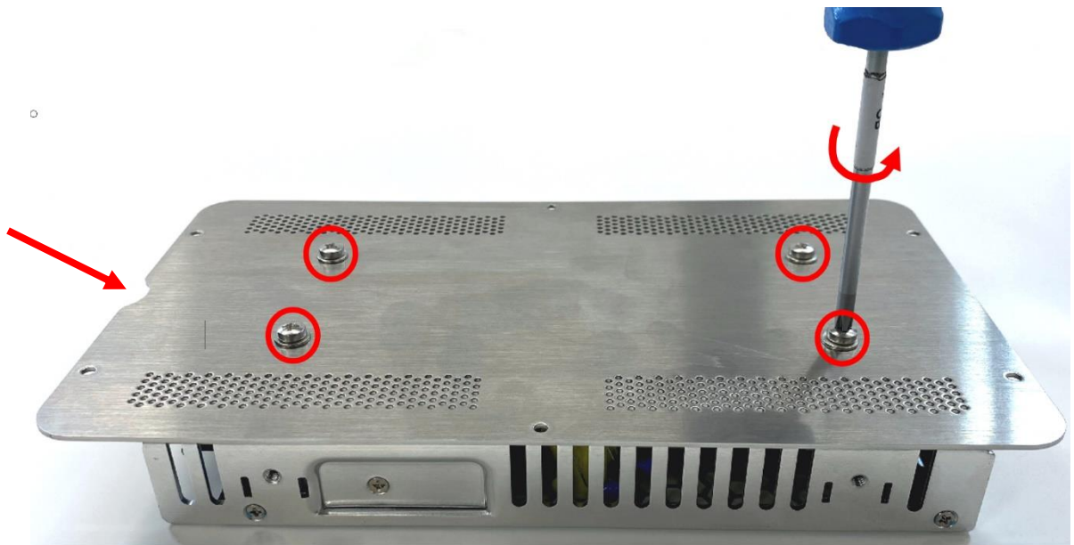
Figure 37. Removing PSU from the PSU frame. The four screws fixing the PSU are encircled in red.
