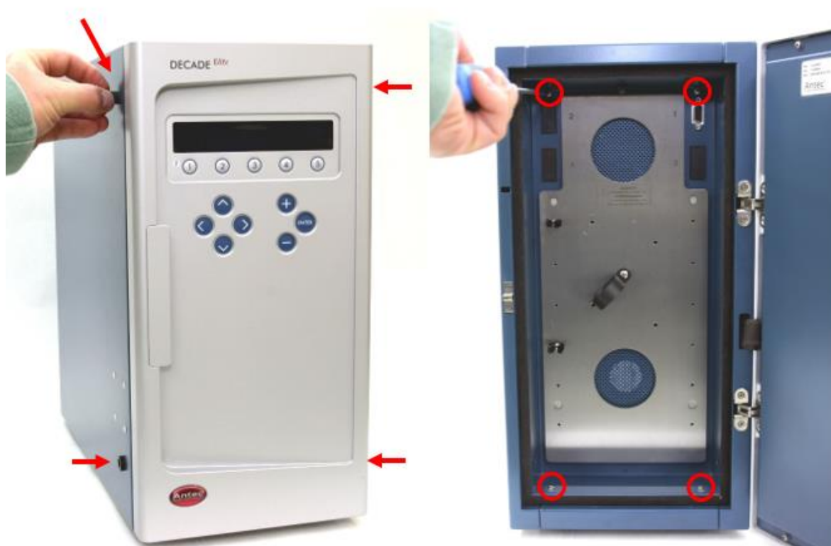
Figure 16. Left: removal of the rubber liners in the inlet/outlet openings in the detector oven compartment. Right: Removing the M3 screws securing the detector cell cabinet.
